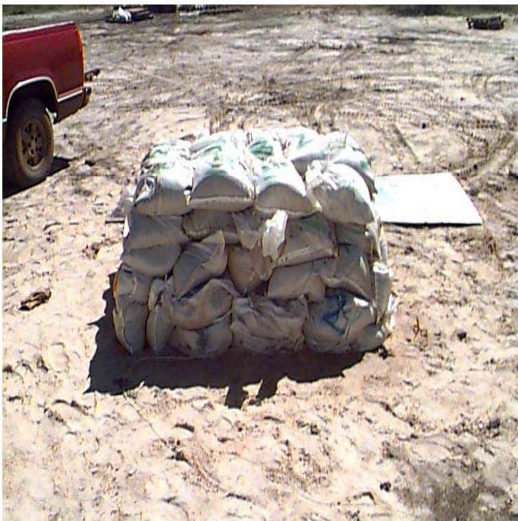
Figure 5 – Sandbag Enclosure for an 81 mm M374A2 mortar.
