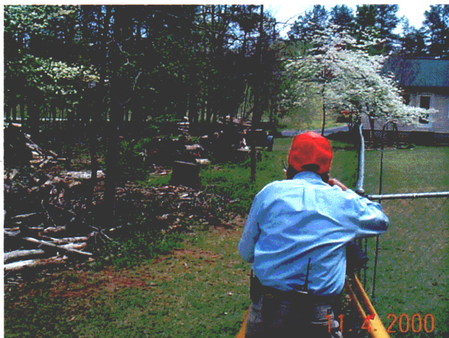
Figure 4: Total Station Measuring System is Not Impacted by the Woods Canopy
