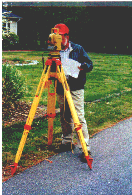
Figure 2: Surveyors Used Electronic Total Station to Stake Anomalies
